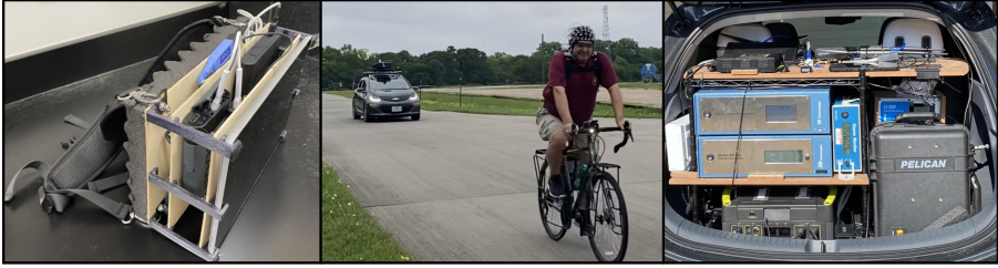
Fig. 7 Data collection images. (Left) Custom made backpack to house biometric devices and recording computer. (Middle) Participant and environmental survey vehicle riding in tandem during data collection. (Right) Environmental sensors organized in trunk of electric survey vehicle.
