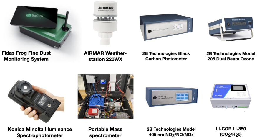
Fig. 9 Images of environmental sensing systems. Fidas® Frog Fine Dust Monitoring System measures particulate matter concentrations at 100 different size bins. The AIRMAR 220WX WeatherStation® Instrument samples barometric pressure, wind speed and direction, ambient temperature, and more. The 2B Technologies Black Carbon Photometer measures atmospheric black carbon particulates using long-path photometry. The 2B Technologies Model 205 Dual Beam Ozone sensor is a UV-based ozone monitor. The Konica Minolta CL-500A Illuminance Spectrophotometer measures the spectral irradiance from 360 to 780 nm at every nanometer. The portable mass spectrometer was constructed by the UNT Laboratory of Imaging Mass Spectrometry and measures charge mass ratios ranging 1 - 300 amu. The 2B Technologies Model 405 nm NO 2 /NO/NO x Monitor™ directly measures atmospheric Nitrogen Dioxide (NO 2 ) and Nitric Oxide (NO). The LI-COR LI-850 Gas Analyzer measured CO 2 and water vapor in the air.
